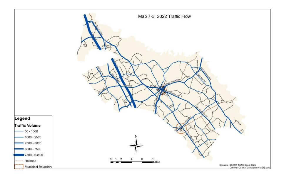
Appendix 7A provides traffic counts for 2012, 2017, and 2022, and the trend established by these counts at each traffic count station in the county is used to develop a least-squares regression forecast for 2045 traffic on each highway segment.
